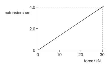
What is the strain energy in the spring when the extension is 4.0 cm?
