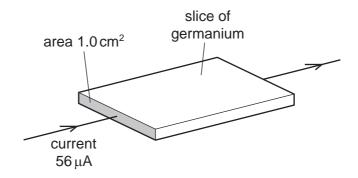
What is the average drift velocity of the charge carriers in the germanium?
