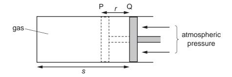
The gas is heated and this causes it to expand, pushing back the piston through distance r from position P to position Q. The length of the gas column is then s.
