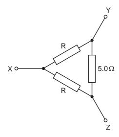
The resistance between Y and Z is found to be  $2.5 \Omega$ .
