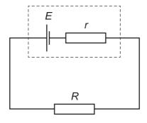
What is the power dissipated in the external resistor?
